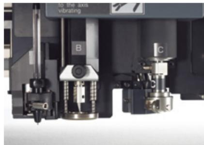
Thick materials up to 20 mm (0.78") can be cut with the reciprocating cutter. The R1 head is equipped with a material-holding unit, which prevents cut materials from lifting. The cutting head is suitable for cutting corrugated boards and foam materials.
