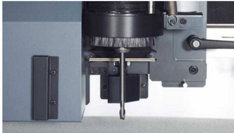
The M head is used exclusively for router cutting. With a high-speed spindle, rigid materials such as acrylic or aluminum composite panels can be cut easily, even up to 50 mm in thickness. The cut depth control function enables multiple cuts for especially thick materials.
